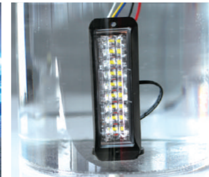
Immersion and pressure Tightness Test
